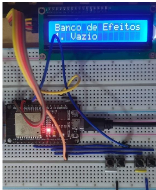
Figura 29: Circuito interface elaborado na protoboard.
