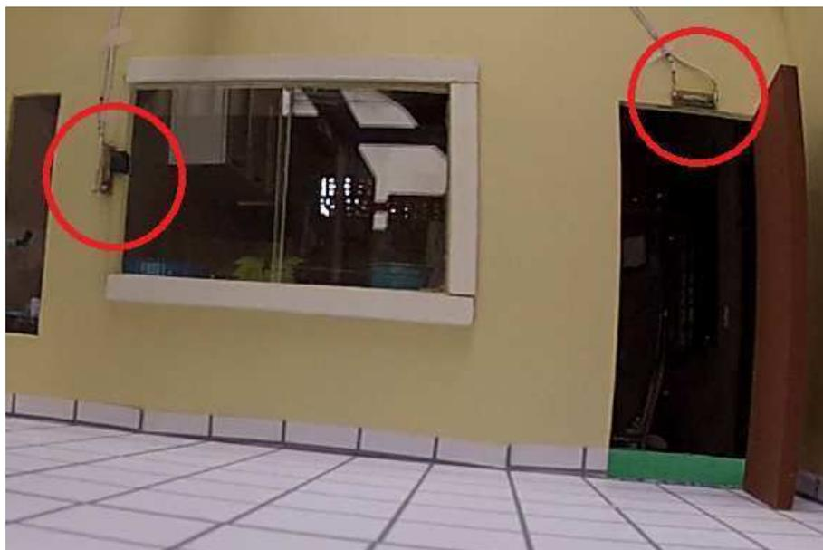
**Figura 42 – Sensores *reed-switches* (maquete).**
