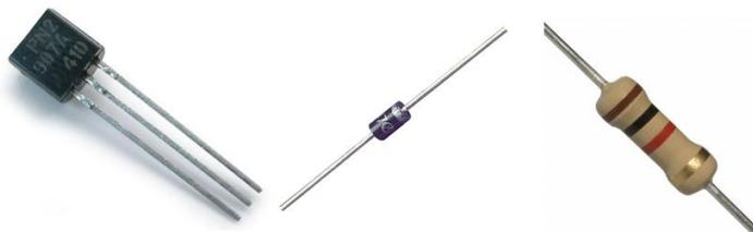
Figura 35 - Transistor NPN 2N3019 / Diodo 1n4007 / Resistor 1K.
